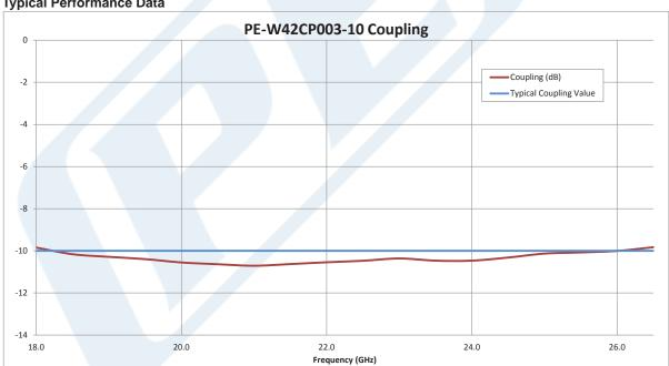
Click the following link (or enter part number in "SEARCH" on website) to obtain additional part information including price, inventory and certifications: WR-42 Waveguide 10 dB Broadwall Coupler, UG-595/U Square Cover Flange, E-Plane Coupled Port, 18 GHz to 26.5 GHz, Brass Copper PE-W42CP003-10
