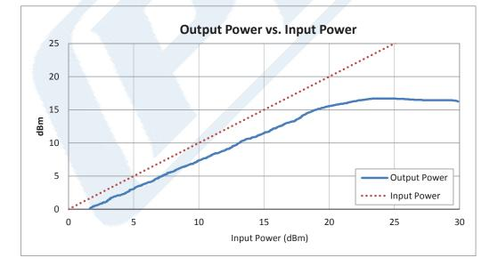
Click the following link (or enter part number in "SEARCH" on website) to obtain additional part information including price, inventory and certifications: High Power Limiter, SMA, 200W Peak Power, 200 us Recovery, 14 dBm Flat Leakage, 2 GHz to 4 GHz PE8031
