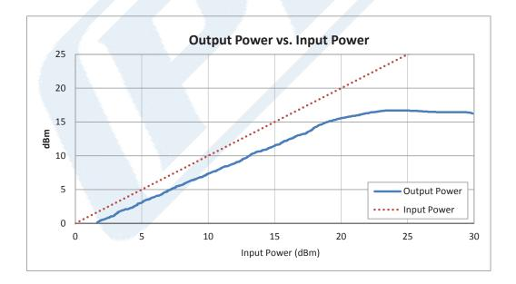
Click the following link (or enter part number in "SEARCH" on website) to obtain additional part information including price, inventory and certifications: High Power Limiter, SMA, 100W Peak Power, 200 us Recovery, 13 dBm Flat Leakage, 4 GHz to 8 GHz PE8034
