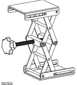
LOAD BEARING CAPACITY OF 40 KG.
