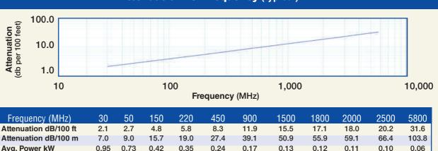
Calculate Attenuation = (0.385082) • √ FMHz + (0.000396) • FMHz (interactive calculator available at http://www.timesmicrowave.com/cable\_calculators)
