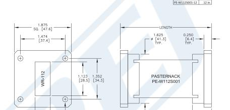
WR-112 Commercial Grade Straight Waveguide Section 3 Inch Length with UG-51/U Flange Operating from 7.05 GHz to 10 GHz from Pasternack Enterprises has same day shipment for domestic and International orders. Our RF, microwave and millimeter wave products maintain a 99% availability and are part of the broadest selection in the industry.
