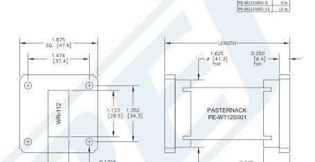
WR-112 Commercial Grade Straight Waveguide Section 9 Inch Length with UG-51/U Flange Operating from 7.05 GHz to 10 GHz from Pasternack Enterprises has same day shipment for domestic and International orders. Our RF, microwave and millimeter wave products maintain a 99% availability and are part of the broadest selection in the industry.
