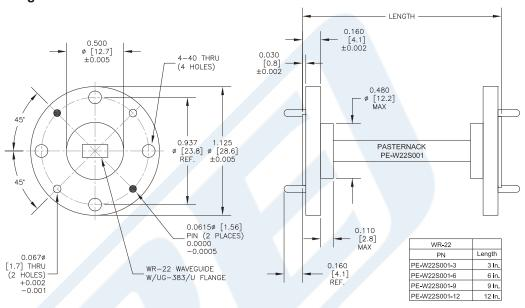
WR-22 Instrumentation Grade Straight Waveguide Section 3 Inch Length with UG-383/U Flange Operating from 33 GHz to 50 GHz from Pasternack Enterprises has same day shipment for domestic and International orders. Our RF, microwave and millimeter wave products maintain a 99% availability and are part of the broadest selection in the industry.
