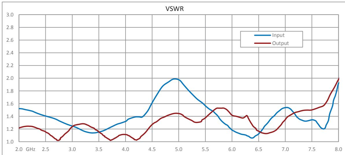
1 Watt P1dB, 2 GHz to 8 GHz, Medium Power Amplifier
