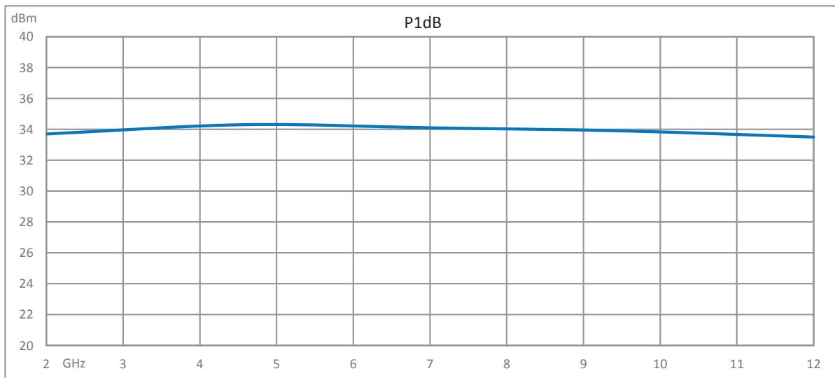
2 Watt P1dB, 2 GHz to 12 GHz, Medium Power Amplifier with Heatsink, SMA, 35 dB Gain, 40 dBm IP3 from Pasternack Enterprises has same day shipment for domestic and International orders. Our RF, microwave and millimeter wave products maintain a 99.4% availability and are part of the broadest selection in the industry.
