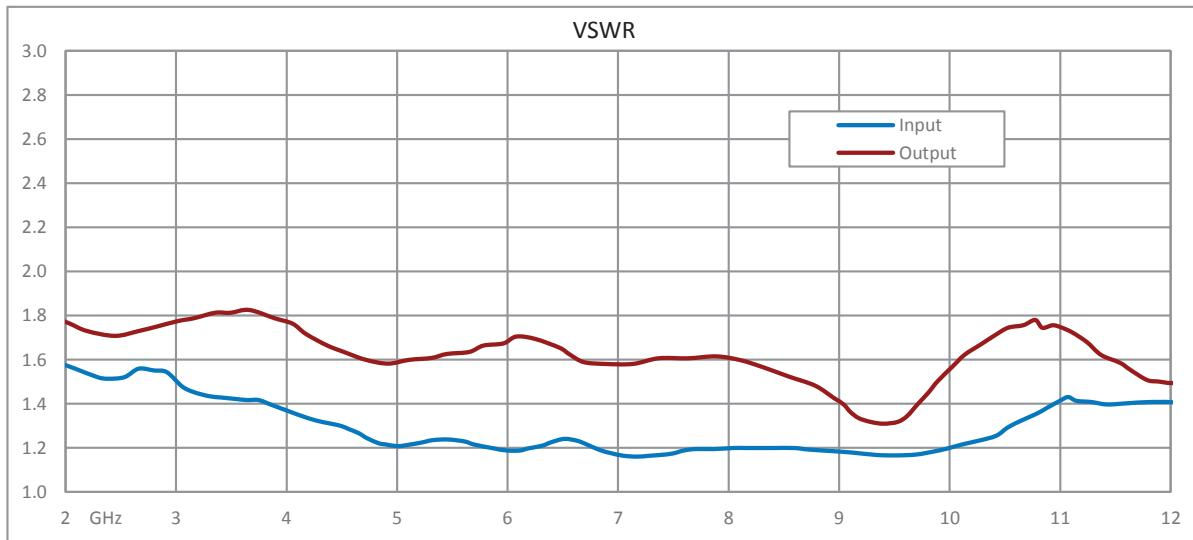
2 Watt P1dB, 2 GHz to 12 GHz, Medium Power Amplifier
