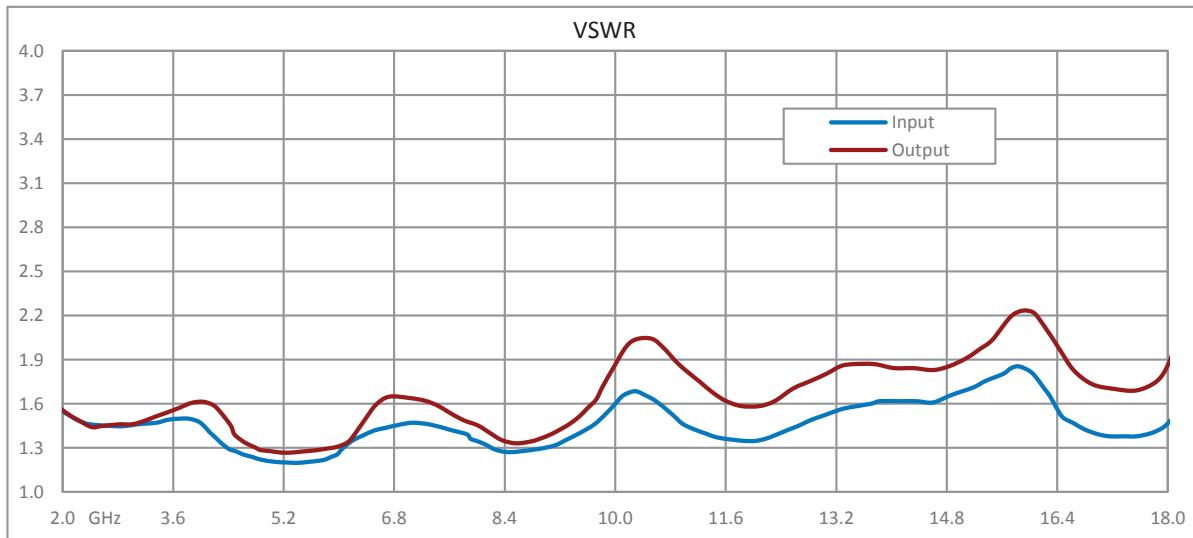
1 Watt P1dB, 2 GHz to 18 GHz, Medium Power Amplifier
