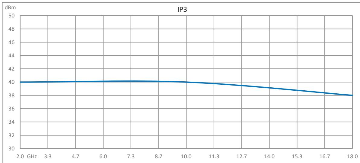
2 Watt P1dB, 2 GHz to 18 GHz, Medium Power Amplifier
