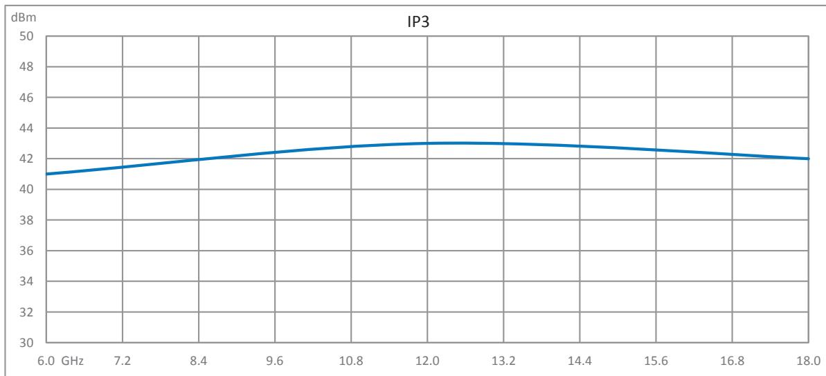
2 Watt P1dB, 6 GHz to 18 GHz, Medium Power Amplifier, SMA, 35 dB Gain, 40 dBm IP3
