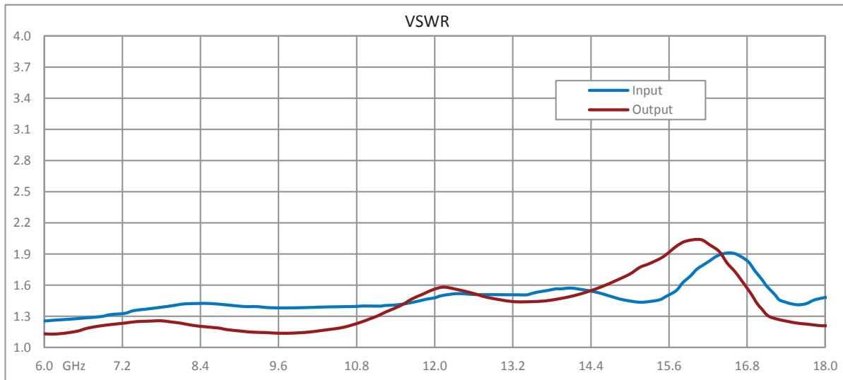
5 Watt P1dB, 6 GHz to 18 GHz, High Power Amplifier
