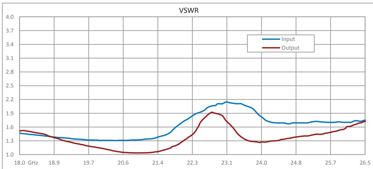
2 Watt P1dB, 18 GHz to 26.5 GHz, Medium Power Amplifier with Heatsink, SMA Input, 2.92mm Output, 35 dB Gain, 40 dBm IP3
