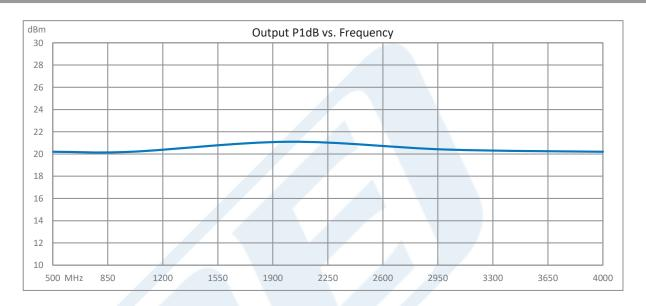
Temperature Compensated Low Noise Amplifier, 0.5 GHz to 4 GHz, 35 dB min Gain, P1dB 20 dBm, SMA from Pasternack Enterprises has same day shipment for domestic and International orders. Our RF, microwave and millimeter wave products maintain a 99.4% availability and are part of the broadest selection in the industry.
