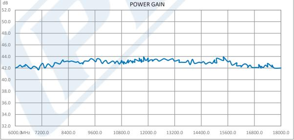
Click the following link (or enter part number in "SEARCH" on website) to obtain additional part information including price, inventory and certifications: 40 dB Gain, 10 Watt Psat, 6 GHz to 18 GHz, High Power GaN Amplifier, Class AB, SMA PE15A5123
