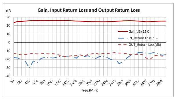
23 dBm P1dB, 50 MHz to 4 GHz, Gain Block Amplifier, 26 dB Gain, 35 dBm IP3, 5 dB NF, SMA from Pasternack Enterprises has same day shipment for domestic and International orders. Our RF, microwave and millimeter wave products maintain a 99.4% availability and are part of the broadest selection in the industry.
