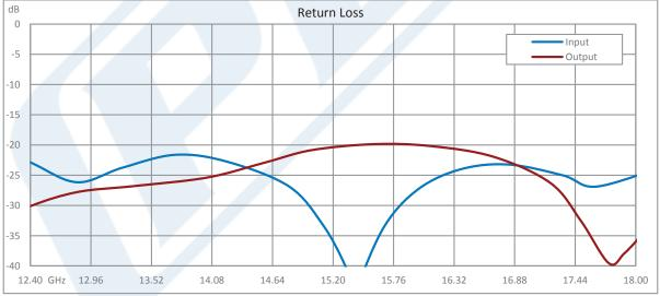
Click the following link (or enter part number in "SEARCH" on website) to obtain additional part information including price, inventory and certifications: Directional 6 dB SMA Coupler From 12.4 GHz to 18 GHz Rated to 4 Watts PE2207-6
