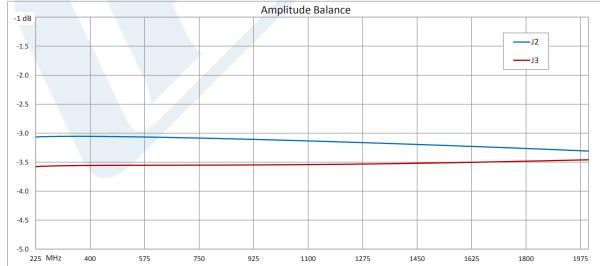
Click the following link (or enter part number in "SEARCH" on website) to obtain additional part information including price, inventory and certifications: 50 Ohm to 25 Ohm Balun From 225 MHz to 2 GHz Up to 100 Watts Surface Mount(SMT) PE2BL1000
