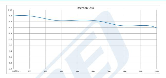
90 Degree Drop-In Hybrid Coupler From 80 MHz to 1,000 MHz Rated to 250 Watts from Pasternack Enterprises has same day shipment for domestic and International orders. Our RF, microwave and millimeter wave products maintain a 99% availability and are part of the broadest selection in the industry.
