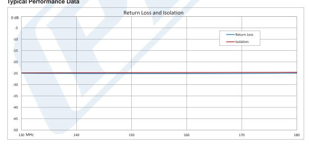
Click the following link (or enter part number in "SEARCH" on website) to obtain additional part information including price, inventory and certifications: 90 Degree Drop-In Hybrid Coupler From 130 MHz to 180 MHz Rated to 200 Watts PE2CP1032
