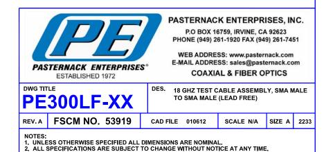
3. DIMENSIONS ARE IN INCHES [mm]. 4. LENGTH TOLERANCE IS  $\pm$  1.5% OR 3/8", WHICHEVER IS GREATER.
