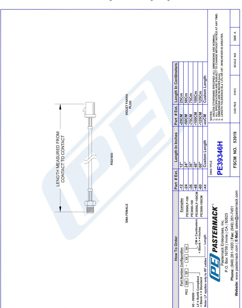
PE39346H-24 CAD Drawing SMA Female to Violet FAKRA Plug Cable 24 Inch Length Using RG316 Coax
