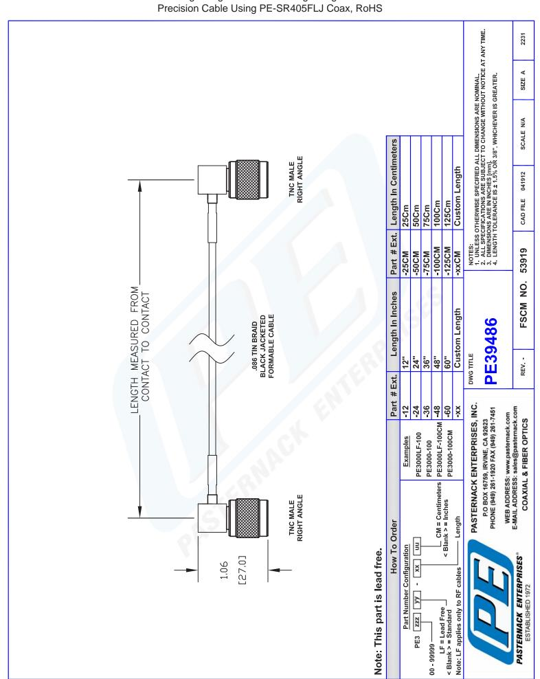
PE39486 CAD Drawing TNC Male Right Angle to TNC Male Right Angle Semi-Flexible
