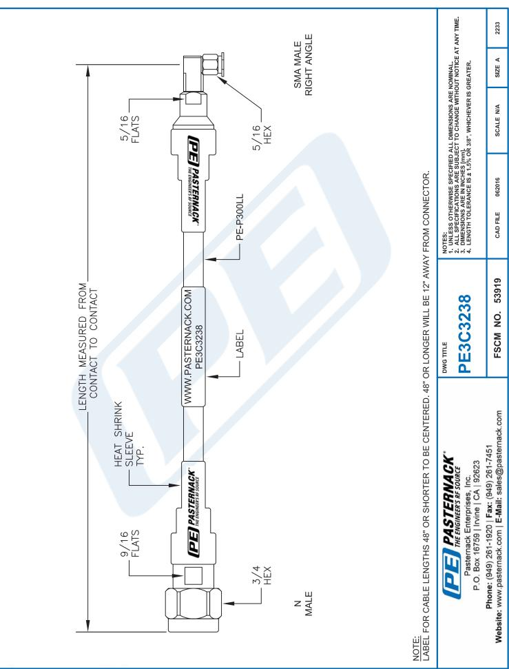
PE3C3238 CAD Drawing SMA Male Right Angle to N Male Low Loss Test Cable Using PE-P300LL Coax, RoHS
