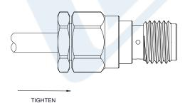
INSERT THE ASSEMBLY INTO THE REAR BODY. HOLD THE NUT STATIONARY AND TIGHTEN THE BODY TO 15 IN LBS.
