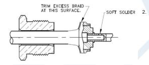
SLIDE CLAMP ASSY OVER DIELECTRIC AND UNDER BRAID UNTIL THE DIELECTRIC BOTTOMS OUT IN CLAMP AND THE CENTER CONDUCTOR IS VISIBLE INSIDE HOLE OF CONTACT. SOLDER THE CONTACT ONTO THE CENTER CONDUCTOR. DO NOT OVERHEAT!.
