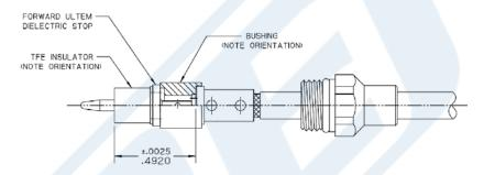
INSERT CABLE/CONTACT SUB-ASSEMBLY INTO CONNECTOR UNTIL SEATED AND TIGHTEN CLAMP NUT TO 35-45 IN-LBS..
