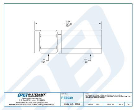
50 Ohm 0.5 Watts Nickel Plated Brass SMC Plug RF Load Up To 1,000 MHz from Pasternack Enterprises has same day shipment for domestic and International orders. Our RF, microwave and millimeter wave products maintain a 99% availability and are part of the broadest selection in the industry.
