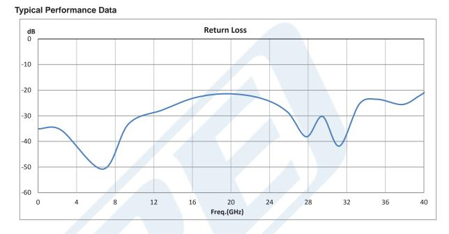
1 Watt RF Load Up to 40 GHz with 2.92mm Female Passivated Stainless Steel from Pasternack Enterprises has same day shipment for domestic and International orders. Our RF, microwave and millimeter wave products maintain a 99% availability and are part of the broadest selection in the industry.
