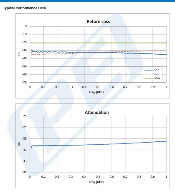
Click the following link (or enter part number in "SEARCH" on website) to obtain additional part information including price, inventory and certifications: 30 dB Fixed Attenuator, 75 Ohm BNC Male to 75 Ohm BNC Female Brass Nickel Body Rated to 1 Watt Up to 1,000 MHz PE7009-30
