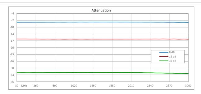
TTL Controlled Programmable Attenuator, 63 dB, from 30 MHz to 3 GHz, 1 dB Steps, SMA Female from Pasternack Enterprises has same day shipment for domestic and International orders. Our RF, microwave and millimeter wave products maintain a 99.4% availability and are part of the broadest selection in the industry.
