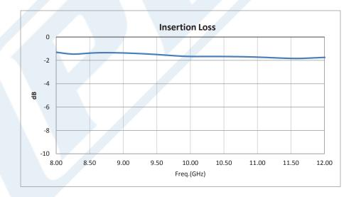
Absorptive SPST PIN Diode Switch Operating From 8 GHz to 12 GHz Up to +20 dBm and Field Replaceable SMA from Pasternack Enterprises has same day shipment for domestic and International orders. Our RF, microwave and millimeter wave products maintain a 99% availability and are part of the broadest selection in the industry.
