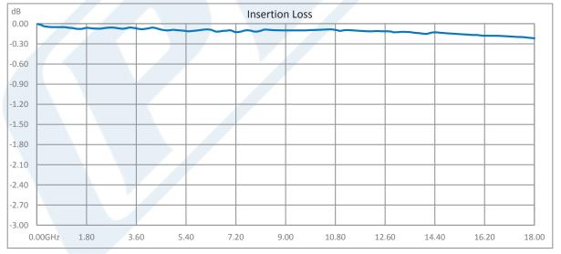
Click the following link (or enter part number in "SEARCH" on website) to obtain additional part information including price, inventory and certifications: SPDT Electromechanical Relay Latching Switch, DC to 18 GHz, up to 90W, 12V, SMA PE71S6352
