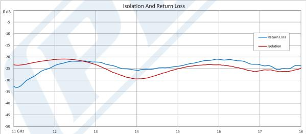
Click the following link (or enter part number in "SEARCH" on website) to obtain additional part information including price, inventory and certifications: High Power Circulator With 20 dB Isolation From 11 GHz to 18 GHz, 50 Watts And SMA Female PE83CR1011
