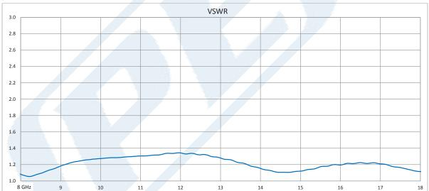
Click the following link (or enter part number in "SEARCH" on website) to obtain additional part information including price, inventory and certifications: High Power Isolator SMA Female with 16 dB Isolation from 8 GHz to 18 GHz Rated to 50 Watts PE83IR1010A
