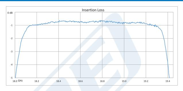
Click the following link (or enter part number in "SEARCH" on website) to obtain additional part information including price, inventory and certifications: 6 Section Bandpass Filter With SMA Female Connectors Operating From 18.2 GHz to 19.2 GHz With a 1,000 MHz Passband PE87FL1009
