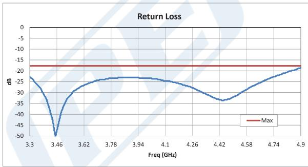
Click the following link (or enter part number in "SEARCH" on website) to obtain additional part information including price, inventory and certifications: WR-229 CMR-229 Flange to N Female Waveguide to Coax Adapter Operating From 3.3 GHz to 4.9 GHz, S-C Band PE9823
