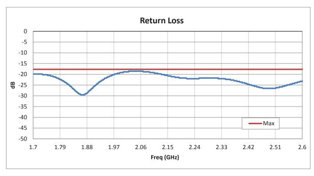
WR-430 CPR-430F Flange to SMA Female Waveguide to Coax Adapter Operating from 1.7 GHz to 2.6 GHz from Pasternack Enterprises has same day shipment for domestic and International orders. Our RF, microwave and millimeter wave products maintain a 99.4% availability and are part of the broadest selection in the industry.
