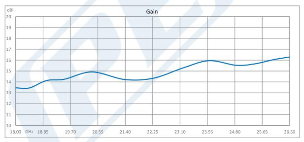
Click the following link (or enter part number in "SEARCH" on website) to obtain additional part information including price, inventory and certifications: WR-42 Waveguide Standard Gain Horn Antenna Operating From 18 GHz to 26.5 GHz With a Nominal 15 dBi Gain With UG-597/U Square Cover Flange PE9852-15
