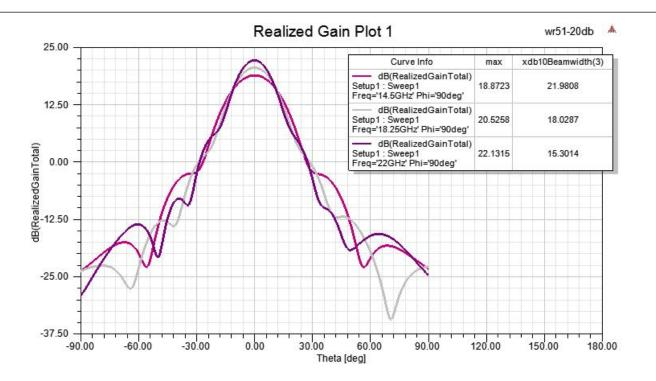
WR-51 Standard Gain Horn with 20 dBi gain, End Launch SMA Female connector from Pasternack Enterprises has same day shipment for domestic and International orders. Our RF, microwave and millimeter wave products maintain a 99.4% availability and are part of the broadest selection in the industry.
