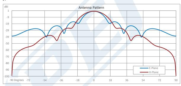
Click the following link (or enter part number in "SEARCH" on website) to obtain additional part information including price, inventory and certifications: WR-15 Waveguide Conical Gain Horn Antenna Operating from 58 GHz to 68 GHz with a Nominal 20 dBi Gain with UG-385/U Round Cover Flange PEWAN1039
