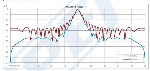
Click the following link (or enter part number in "SEARCH" on website) to obtain additional part information including price, inventory and certifications: WR-15 Waveguide Lens Horn Antenna Operating from 55 GHz to 65 GHz with a Nominal 32 dBi Gain with UG-385/U Round Cover Flange PEWAN1077
