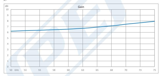
Click the following link (or enter part number in "SEARCH" on website) to obtain additional part information including price, inventory and certifications: WR-15 Waveguide Probe Antenna Operating from 50 GHz to 75 GHz with a Nominal 6.5 dBi Gain with UG-385/U Round Cover Flange PEWAN1128
