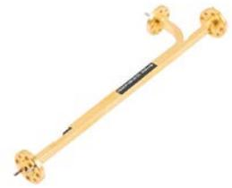
WR-15 Waveguide 20 dB Broadwall Coupler, UG-385/U Round Cover Flange, E-Plane Coupled Port, 50 GHz to 75 GHz, Brass Copper
