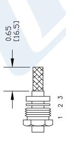
2. FORM BRAID OVER CLAMP NUT (4).TRIM BRAID BACK CONDUCTOR TO DIMENSION SHOWN. DO NOT NICK CENTER CONDUCTOR. TIN CENTER CONDUCTOR SLIDE ASSEMBLY INTO BODY, SOLDER CENTER CONDUCTOR IN PLACE, TIGHTEN CLAMP NUT & TO SHOULDER. CUT DIELECTRIC & CENTER SCREW CAP
