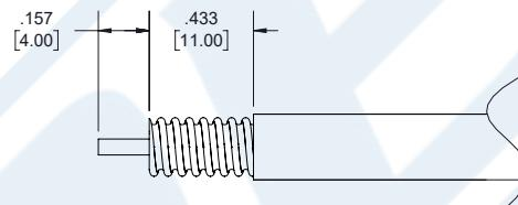
2. SLIDE INSULATOR (3) OVER CABLE CENTER CONDUCTOR. INSERT CENTER CONTACT AND SOLDER. WRAP THE CABLE BY SOLDER WIRE.
