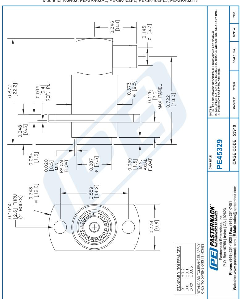
BMA Jack Right Angle Slide-On Connector Solder Attachment 2 Hole Flange Mount for RG402, PE-SR402AL, PE-SR402FL, PE-SR402FLJ, PE-SR402TN
