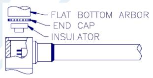
5. PRESS INSULATOR AND END CAP INTO CONNECTOR BODY AND USE A FLAT BOTTOM ARBOR TO PRESS CAP IN PLACE. CAP MUST BE BELOW BODY SURFACE TO SEAT PROPERLY.
